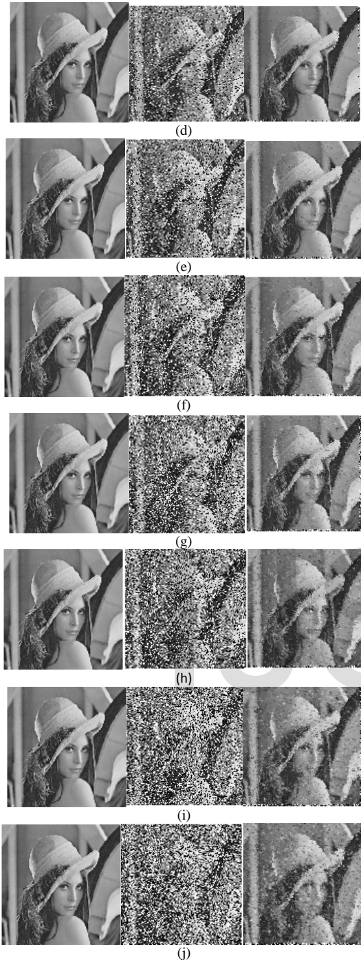
Fig.8 Proposed noise removal filter output for Lena image corrupted by (a)5% (b)10% (c)15% (d)20% (e)25% (f)30% (g)35% (h)40% (i)45% (j)50% noise densities.
